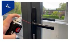
Use a light machine oil on moving handle parts, but not the lock cylinder
